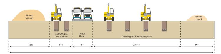
NB: Numbers in brackets are 'worst case' based on conductor size of 1400mm² and burial of between 3.5m to 4.0m
